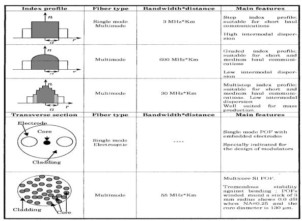
Fig. 3: Types of refractive index profiles in POFs and their main features.
