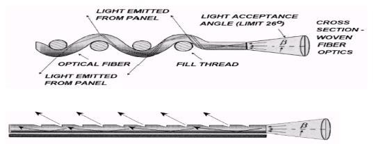
Fig. 5: POF in weaving emits light, and fabric with light emission can be made, or alternatively the surface may have an abraded construction
